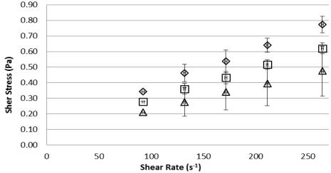
Figure 1 Rheograms for shear stress versus shear rates plots of koumiss at various temperatures  $4^{\circ}\text{C}$  ( $\Diamond$ ),  $10^{\circ}\text{C}$  ( $\square$ ), and  $20^{\circ}\text{C}$  ( $\Delta$ )
