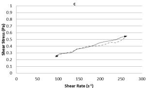
Figure 2 Thixotropic hysteresis curves for koumiss at 4°C (a), at 10°C (b), at 20°C (c)
